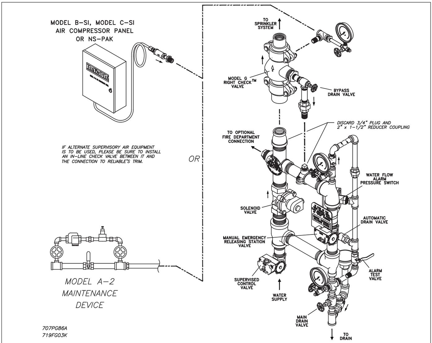
Figure 3 — Single Interlock Preaction, Component Identification
