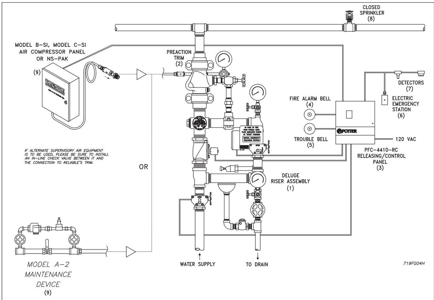
Figure 4 — Single Interlock Preaction System
