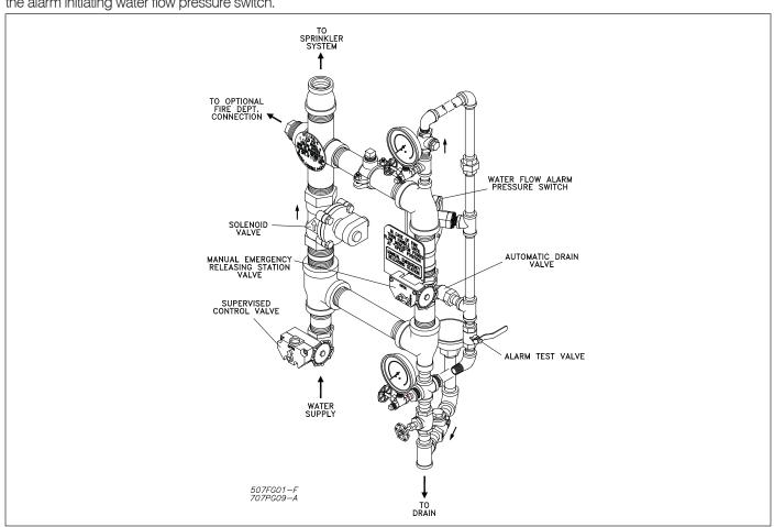
Figure 1 - Model H Deluge Riser Assembly
