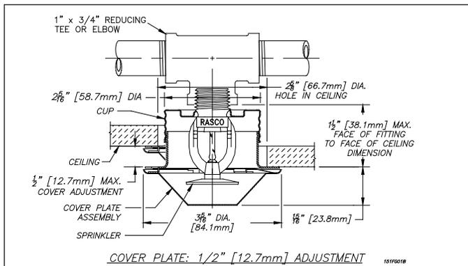
the ceiling surface. Cover plate removal requires turning in the counter clockwise direction.
