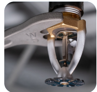
W5 wrench locks into sprinkler boss
