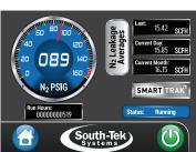
Monitor current N2 pressure and leakage trends in realtime.
