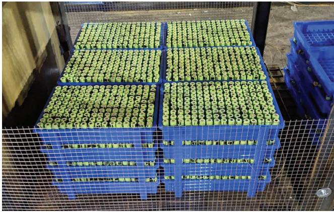
Figure 3: Trays Loaded with Lithium-Ion Batteries
