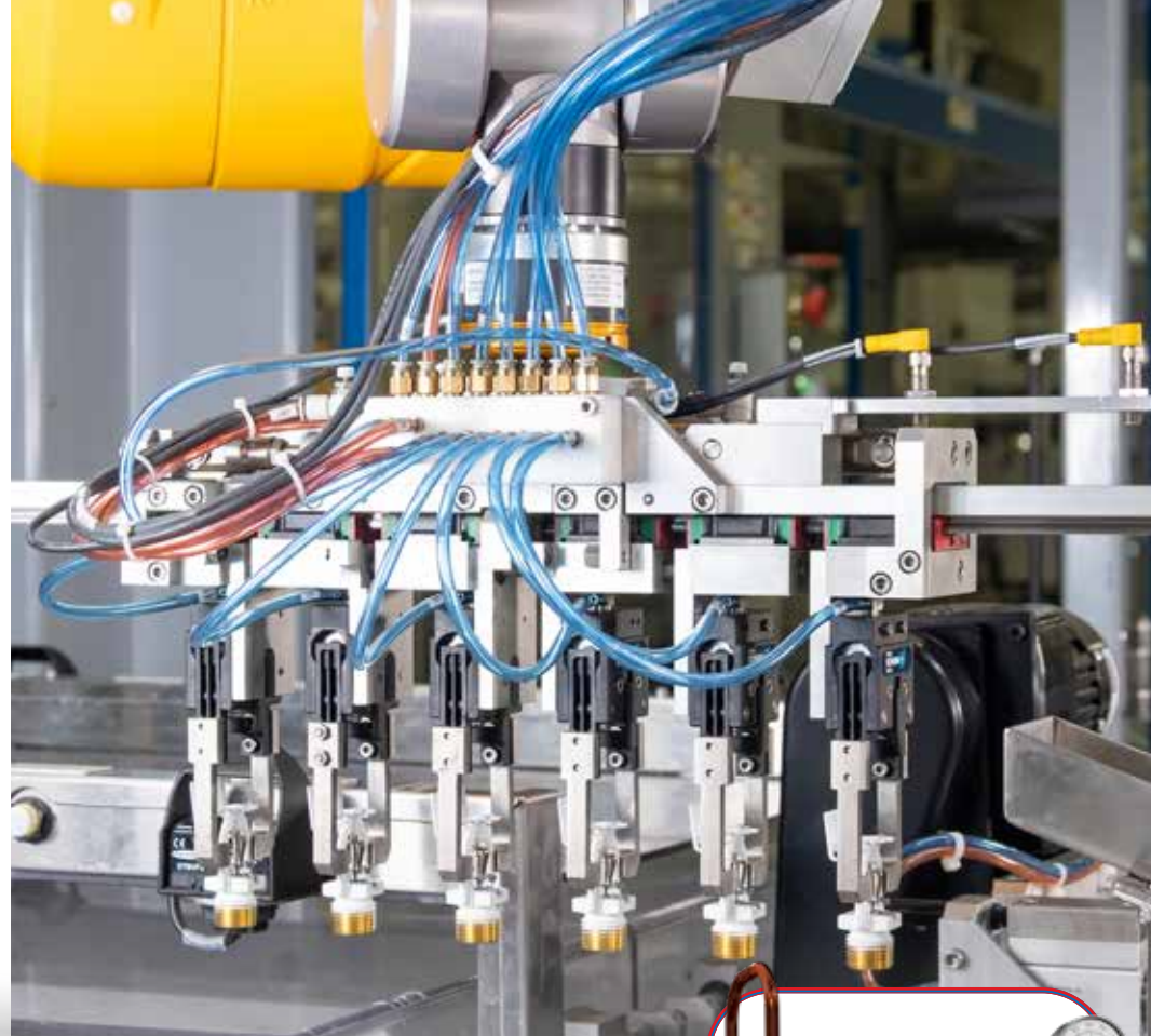
Automated assembly of KFR Series Sprinklers (2019)
