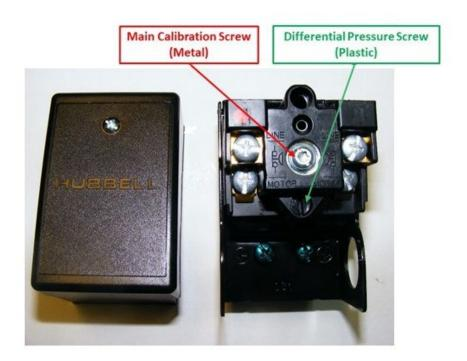
QRM2- Models <u>with</u> Tank (RASCO Part Number 6990028654) Factory Set at 60 PSIG Cut-IN / 80 PSIG Cut-OUT QRM2- Models <u>without</u> Tank (RASCO Part Number 6990021904) Factory Set at 20 PSIG Cut-IN / 26 PSIG Cut-OUT
