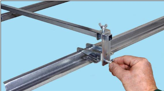
4. Tighten the wing screws, M6 x 1-3/4” located at the bottom of each hat channel side bracket to an approximate torque of 40 inch-lbs, approximately 1/2 to 3/4 turn past hand tight.
