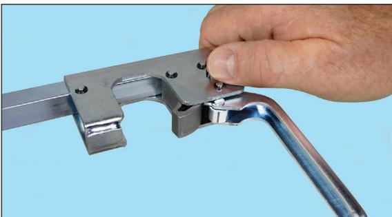
3. Pull the handle towards the installer to open the Gate of Center Bracket.
