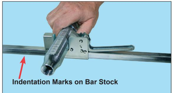
8. When both side brackets are securely attached onto the grid, open the Center Bracket gate and insert the Reducer portion of Flexible Hose to the gate. Adjust height of Reducer to desired position. For center of tile installations, position the center bracket between the two indentation marks on the bar stock as shown above.
