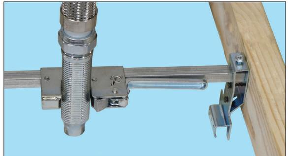
8. Place the outlet reducer into the center bracket, then adjust the height of the outlet reducer to the desired level and lock the reducer into place by closing the handle on the center bracket firmly until you hear click sound. While doing so, use other hand to hold the bar stock to minimize the movement caused by closing the handle.
