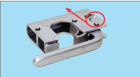
1. Look for the Ring-Shaped Wire Hook located at the top right corner of the Center Bracket
