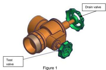
Testing with this valve gives the advantage that the valve clapper can also be tested.
