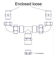
Retrofit kit for 2 pressure switches Part no. 6999996232
