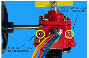
2. When removed, each silver-colored outer set screw will reveal a dark-colored second inner set screw underneath. The inner set screw is the one that serves to adjust the mechanical stop; once set the outer set screw is used to lock the inner set screw in place through friction and keep the inner set screw from vibrating loose. In the figure below, the outer set screw has been removed and the inner set screw can be seen at the bottom of the threaded set screw hole.
