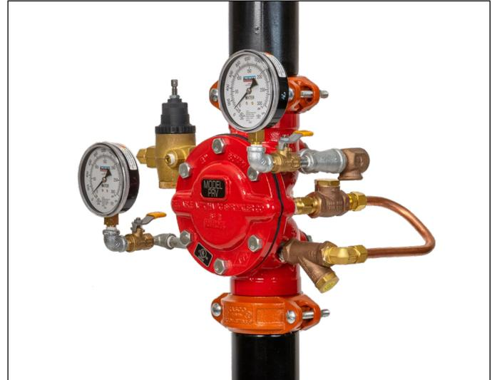
Maintenance of the valve is simplified because all trim is connected to the valve body, and the diaphragm can be removed without disassembling the trim.
