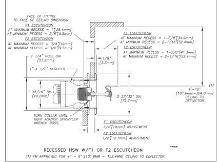
**Note:** For Recessed HSW Sprinklers use installation wrench W4. FM and cULus permits use with F1 or F2 escutcheons for "Light Hazard" only.
